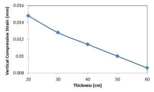
Figure 3. Relationship between the thickness of base course layer and vertical compressive strain at the top of subgrade layer (9% lime)
