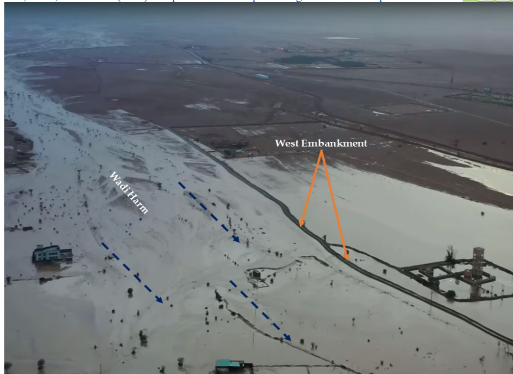
Fig. 29: the impact of Wadi Harm floods on the city of Al Bidi, which indicates the Embankment that directed the water into the city with a negative effect on 18/07/2021
