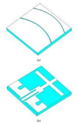
Fig. 1. (a) Back view and (b) Front view of the simulated CST design of the proposed low pass filter.
