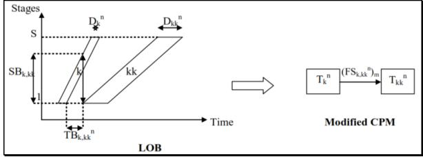
Figure 1: Modified CPM Integrated with LOB when Critical Stage is First Stage
