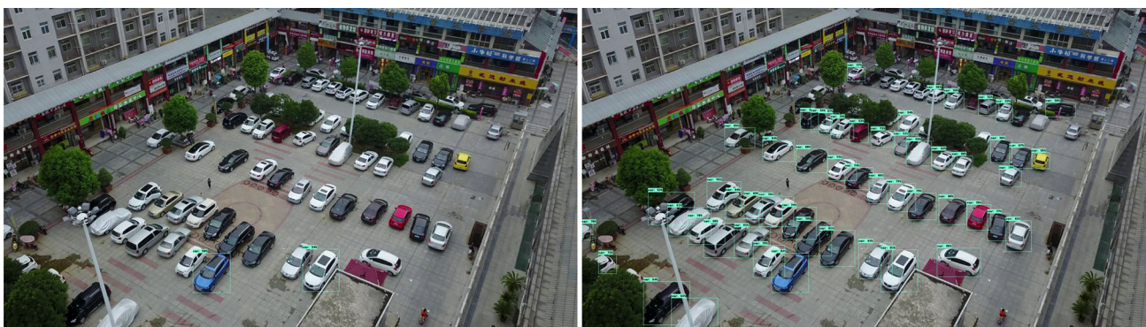
Fig. 8 Frame 0000001_05499_d_0000010 of the VisDrone dataset [32] processed by EfficientDet D4 with a confidence > 50%. The left side shows the results obtained by the raw model, while the right side shows the detections after applying our optimized proposal with R = 50\%
