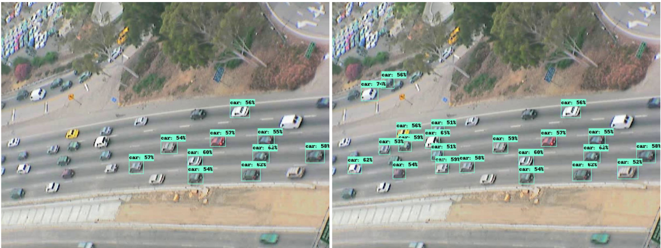
Fig. 5 Frame 3 of the first video denoted as sb-camera1-0820am-0835am processed by CenterNet HourGlass 104 Kpts with a confidence > 50\% . The left side shows the results obtained by the
