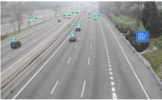
Fig. 3. An example applied to frame 401 of the M30-HD sequence [27]. The left side shows the results of the Fine Tune with the raw model, while the right side shows the detections after applying the Fine Tune with the outputs of the described technique using sequence three and the EfficientDet D4 model.
