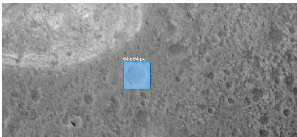
Fig. 7 Selection of region from the DEM of a crater. The elevation used is half of the original. Preparation of the map used for the simulation tests with the anisotropic planner. It is based on the shape of a real crater on the Martian surface. The resolution of the DEM is 1 m
