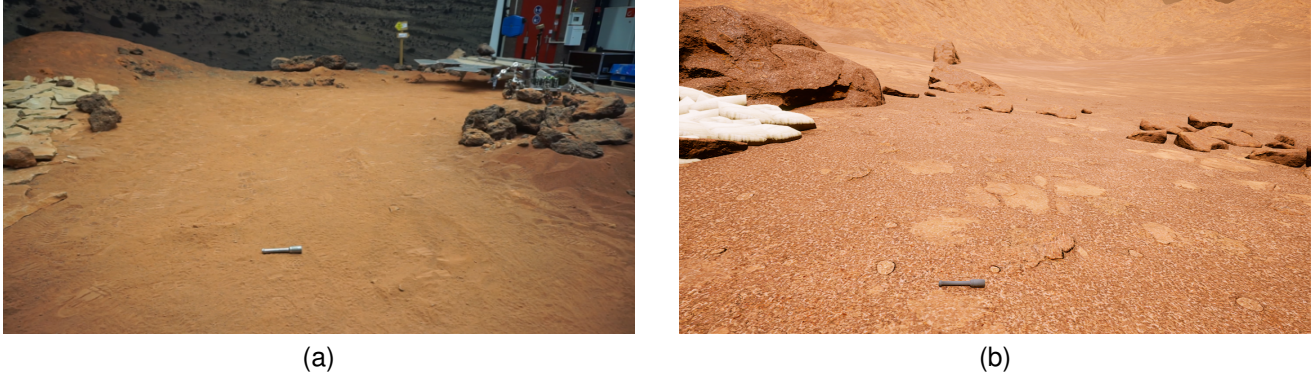
Fig. 6. Figure (a) shows the sample tube on sandy terrain in the ESA's PUTB. Rocks of several sizes are observed on the background. Picture (b) depicts the sample tube in an Unreal Engine 4 simulation. Rocks and obstacles produce shadows depending on a virtual sun position.
