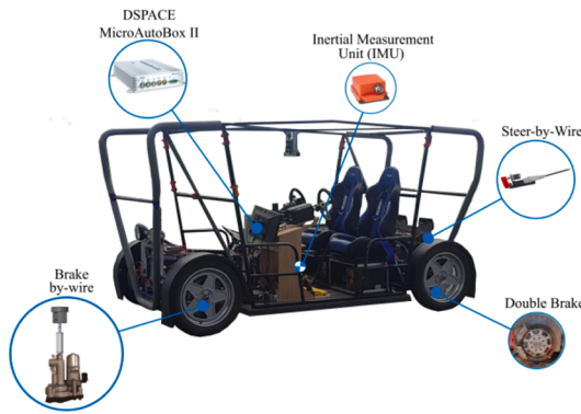
Fig. 14. Research concept vehicle model E (RCV-E) (Left) and electro-hydraulic proportional brake system (right).
