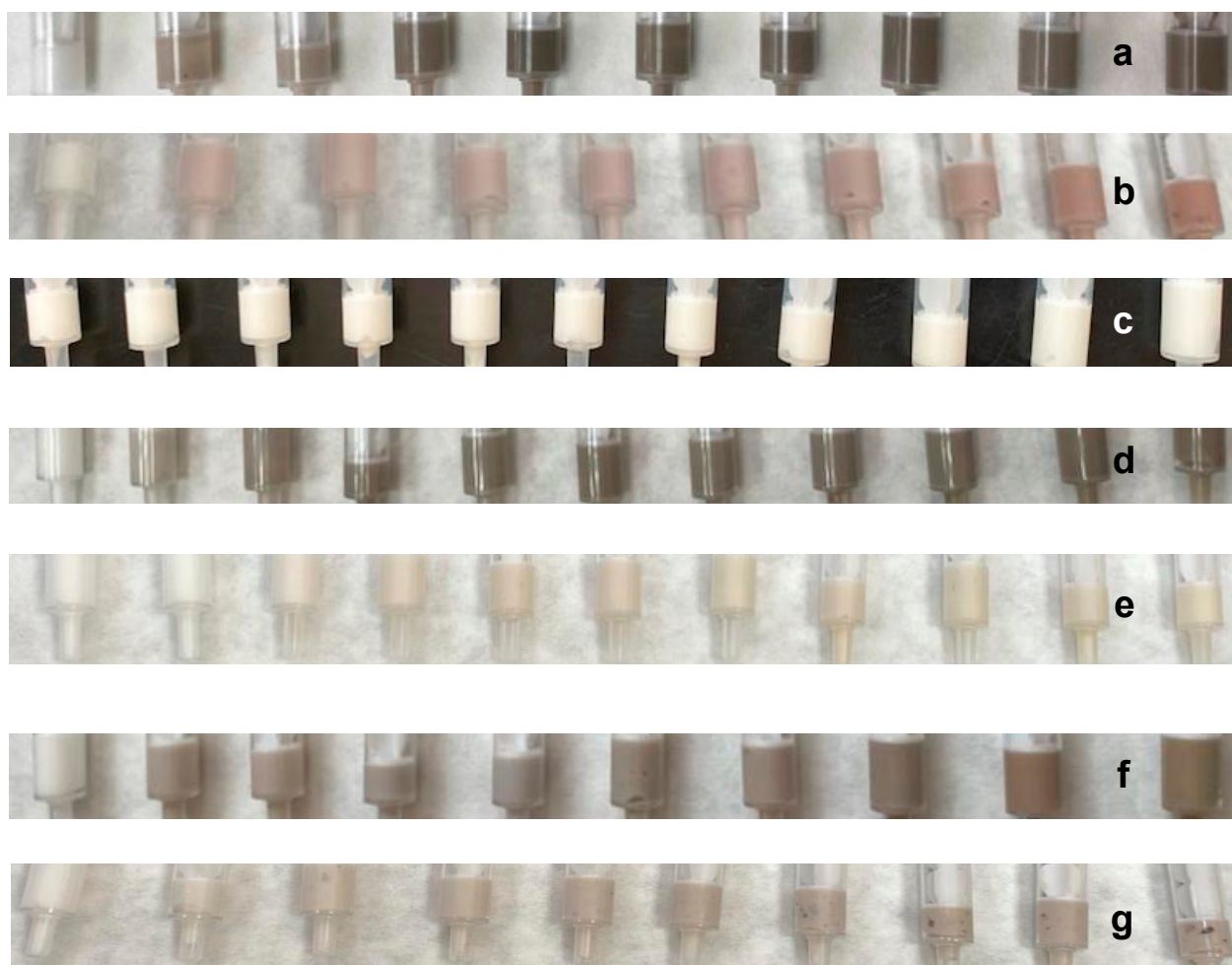
Figure 6. Body creams (1.0 g) prepared with (a) AgNPs (blank, 0.1, 0.2, 0.3, 0.4, 0.5, 0.6, 0.7, 0.8 and 0.9 mg), (b) PCE (blank, 0.1, 0.2, 0.3, 0.4, 0.5, 0.6, 0.7, 0.8 and 0.9 mg), (c) PCE after two days from addition, (d) AgNPs/PCE (blank, 0.1/1.0, 0.2/2.0, 0.3/3.0, 0.4/4.0, 0.5/5.0, 0.6/6.0, 0.7/7.0, 0.8/8.0, 0.9/9.0 and 1.0/10.0 mg), (e) PCE encapsulated in \beta CD (blank, 1.0, 2.0, 3.0, 4.0, 5.0, 6.0, 7.0, 8.0, 9.0 and 10.0 mg), (f) AgNPs and PCE encapsulated in \beta CD (blank, 0.1/1.0, 0.2/2.0, 0.3/3.0, 0.4/4.0, 0.5/5.0, 0.6/6.0, 0.7/7.0, 0.8/8.0 and 0.9/9.0 mg), and (g) PCE encapsulated in p NIPAM (blank, 1.0, 2.0, 3.0, 4.0, 5.0, 6.0, 7.0, 8.0, 9.0 and 10.0 mg). All images show increased concentration from left to right.
