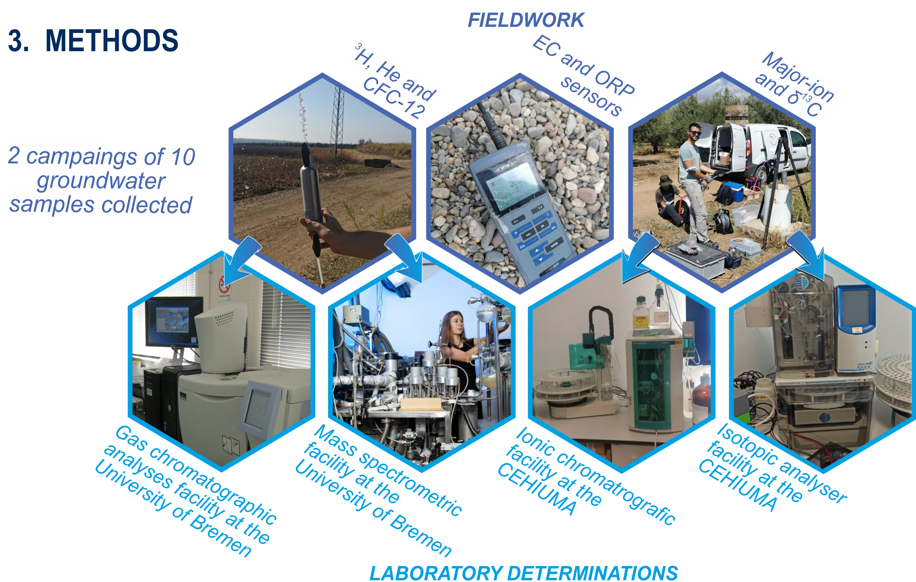
Fig. 2. Methodology applied during the groundwater sampling campaigns carried out and the analysis of water samples taken. Electrical conductivity -EC-; Oxidation Reduction Potential -ORP-
