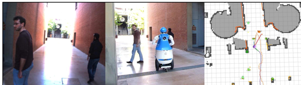
Figure 10. The robot Dabo accompanying a person to the desired goal while navigating in a crowded scenario [74]: (left) image captured from the robot camera; (center) the robot Dabo; (right) the robot GUI. The green cylinders correspond to people and the orange cylinder corresponds to the target. Permission by ELSEVIER 5483750554512.
