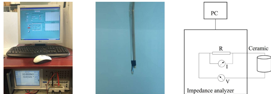
Figure 9. Experimental setup and schematic diagram for impedance measurement.
