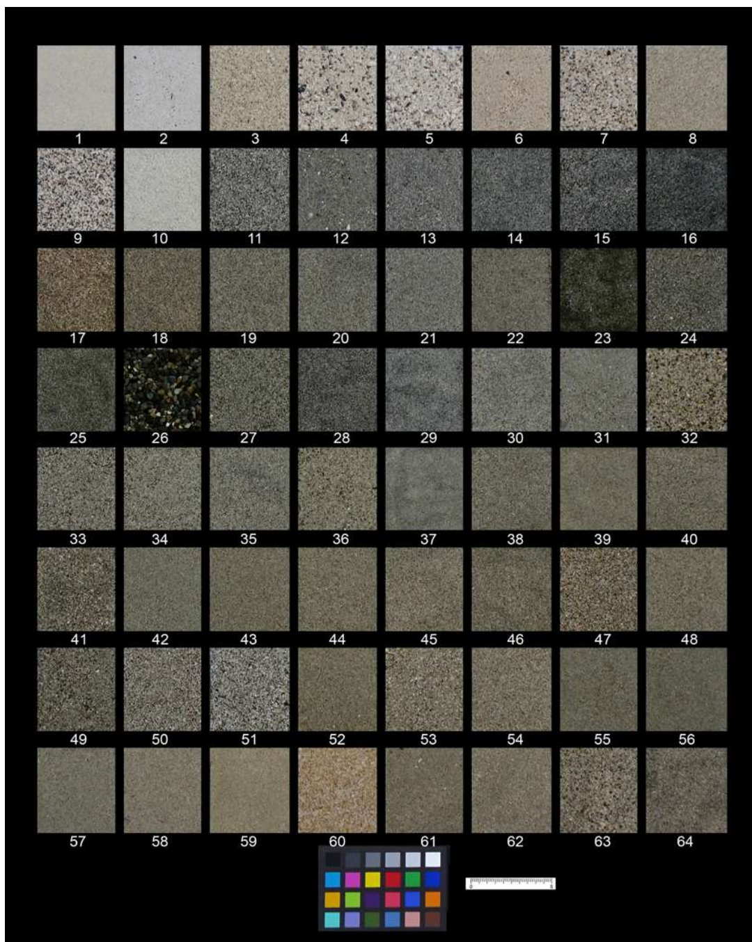
Figure 3. The 64 beach sand samples collected in the Galapagos (1–10) and on the mainland coast (11–64) of Ecuador. Single photo shoot capturing all the samples in order to have the same illumination. X-rite color checker for calibration.
