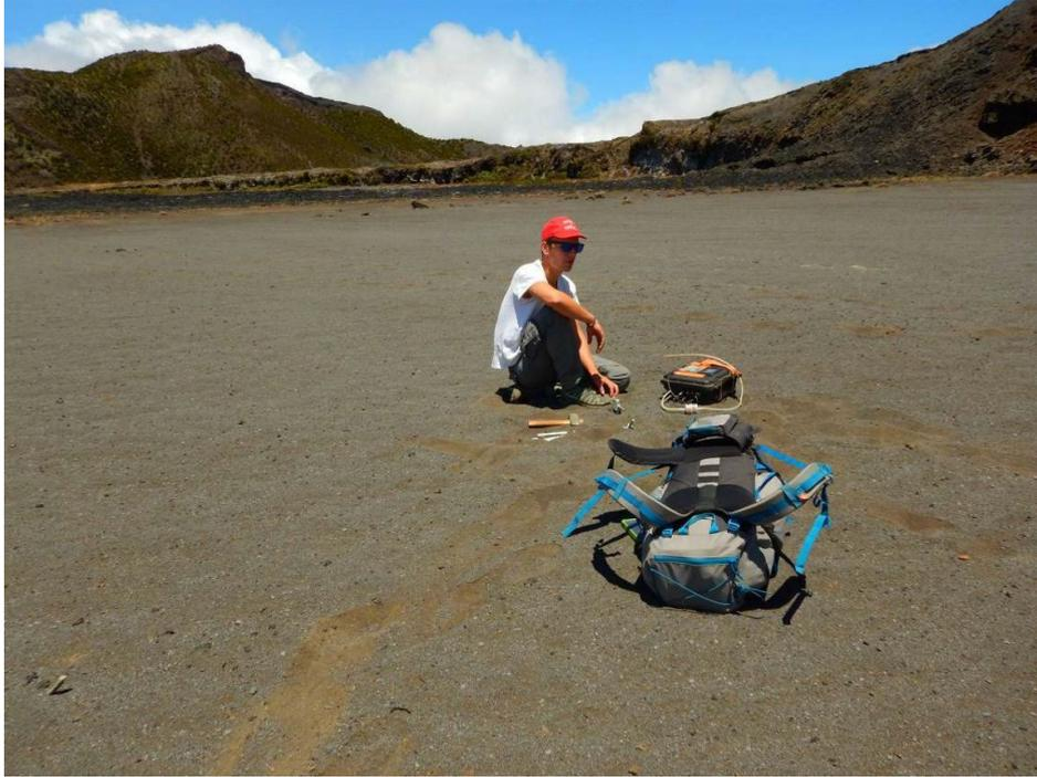
Figure 8. Sampling soil CO<sub>2</sub> gas by the dynamic method in the Karthala summit area
