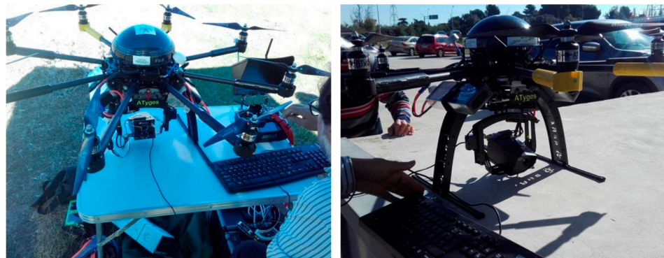
Figure 1. Images of the drone used for the aerial IR thermographic inspection.
