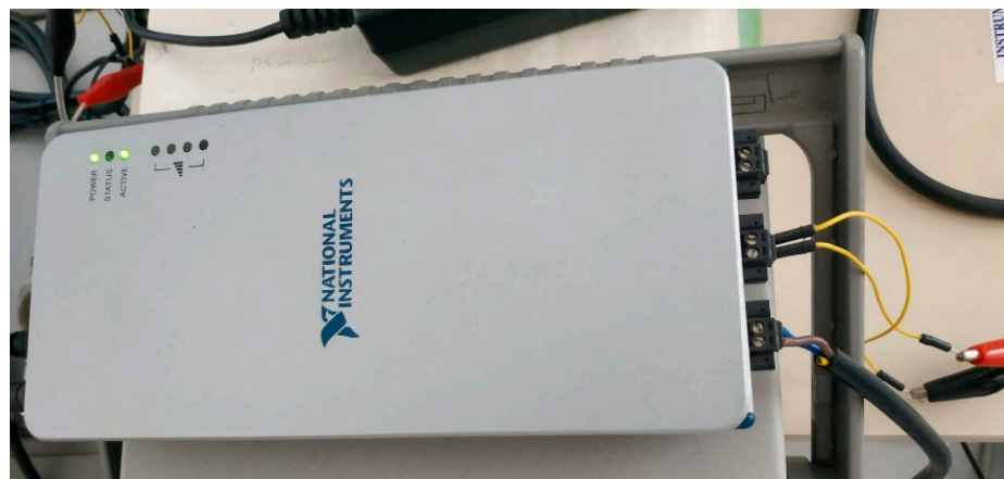
Figure 3. The NI 9225 card inside the chassis cDAQ-9191 (1-Slot, Ethernet and 802.11 Wi-Fi compact DAQ chassis) with wiring connections: Yellow wires (“crocodile”-type probes) correspond to the GPS-PPS signal while the black-covered wires brings the network voltage signal directly by connecting to it with a plug.
