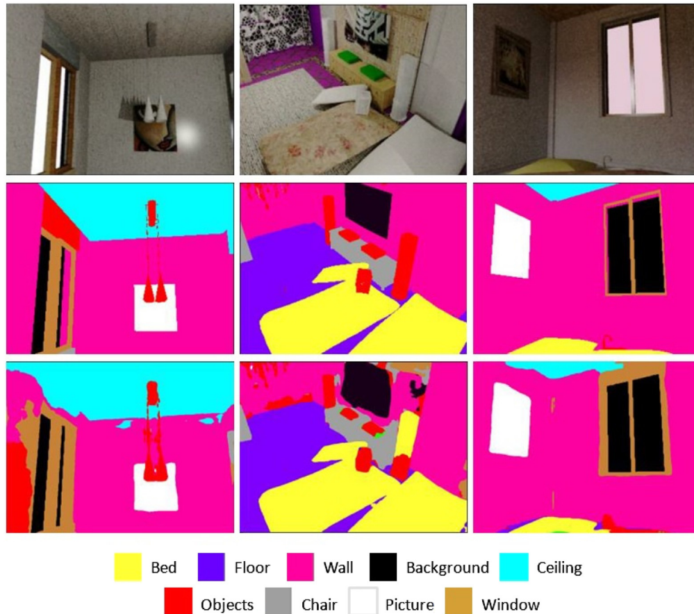
Fig. 6 Segmentation samples on the validation set of the SceneNet dataset (top row: RGB image, middle row: ground truth, and last row: predictions).
