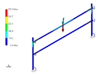
Figure 10. FEA von Mises stress in tests 7 and 8 for reference material (GS).
