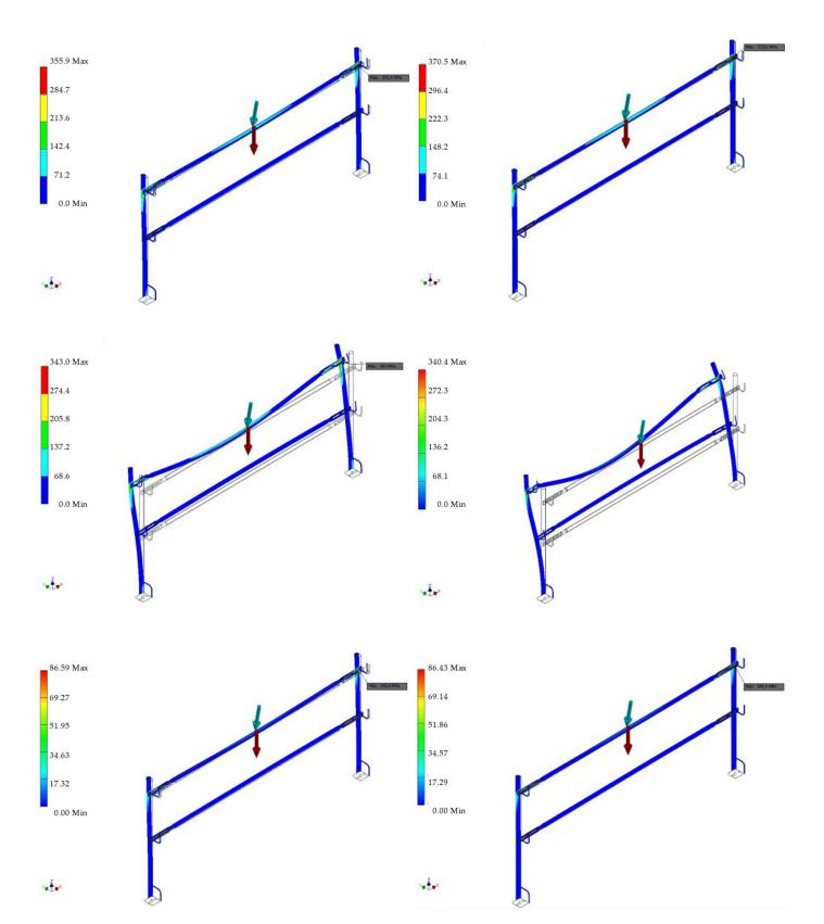
**Figure A5.** FEA von Mises stress in tests 7 and 8 for alternative materials: AL (**top left**), CI (**top right**), PET (**centre left**), PVC (**centre right**), GRFP (**bottom left**) and CRFP (**bottom right**).
