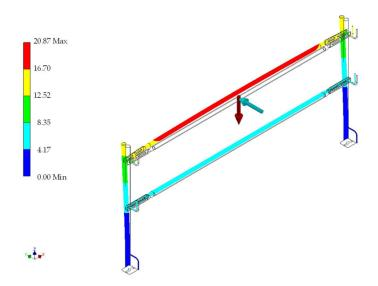
Figure 6. FEA deflection in test 1 for reference material (galvanised steel).
