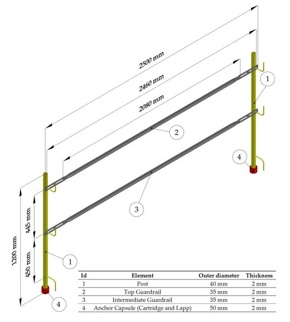
Figure 4. Description of the set of traditional elements (upright and horizontal railing) used as TEPS.
