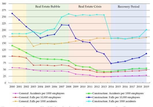
**Figure 2.** Accidents caused by falls from height in the construction sector and in all economic sectors (in general). Source: INE.
