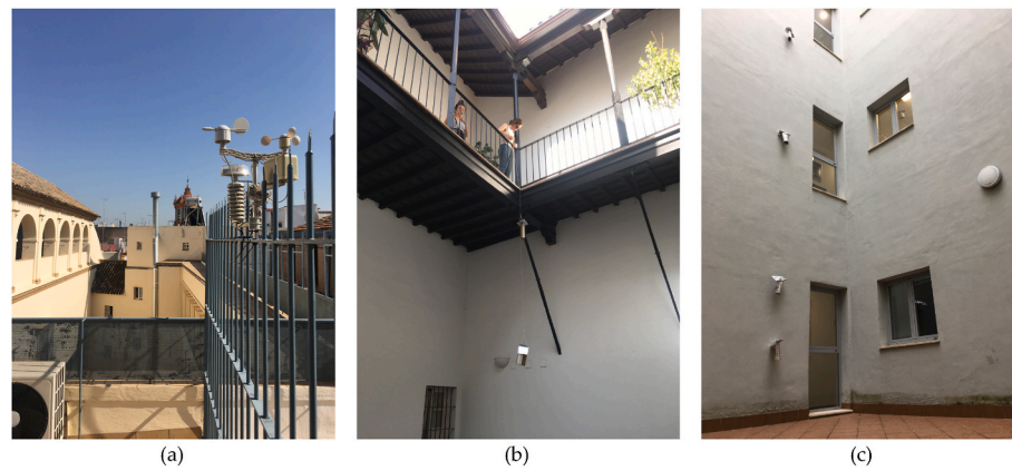
Fig. 3. Location of the measurement instruments. a) wather station PCE-FWS 20, b-c) data loggers TESTO 174 in CS2 (b) and CS3 (c).
