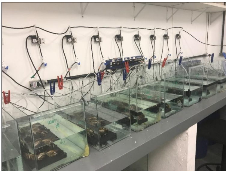
Figure 1: Image of the CO 2 injection system used in this study for the adult mussel's exposition to crack-cocaine in different pHs.
