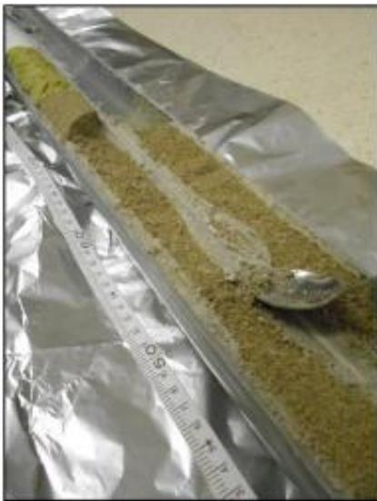
Fig. 4 Sampling sand from inside the tube corer
