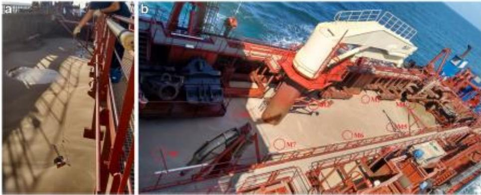
Fig. 3 a. Van Veen grab (spoon) sampler, b. Location of the 8 eight points where superficial samples were taken, named as M1... M8
