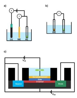
**Figure 2.** Scheme of main transduction mechanisms for lactate electrochemical (bio)sensors: amperometric (**a**); voltammetric (**b**) and field-effect transistor (**c**).
