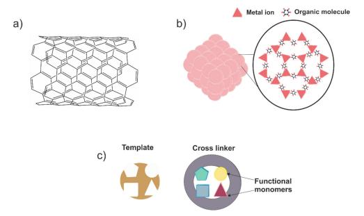
**Figure 4.** Main alternate approaches to enzyme-based lactate sensors: (**a**) nanomaterials, (**b**) metalorganic frameworks (MOFs) and (**c**) molecularly imprinted polymers (MIPs).
