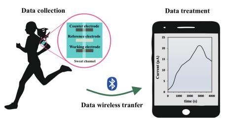
**Figure 5.** General scheme of the performance of a wireless wearable lactate amperometric biosensor for sweat monitoring.
