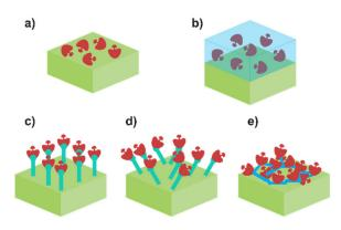
**Figure 3.** Scheme of different enzyme immobilisation approaches: (**a**) adsorption, (**b**) physical entrapment, (**c**) oriented covalent binding, (**d**) random covalent binding and (**e**) crosslinking methods.
