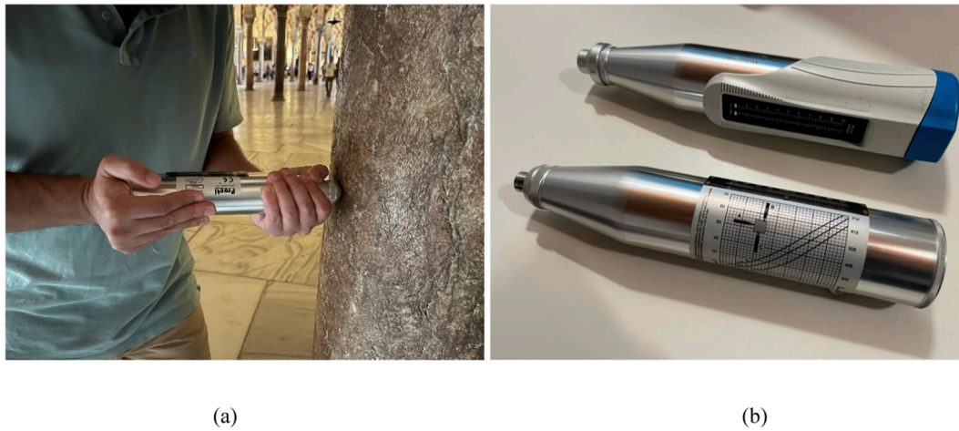
Fig. 8. (a) Performing the Schmidt Hammer test on columns of the sector. (b) Schmidt Hammer devices used for the stone and for the masonry.
