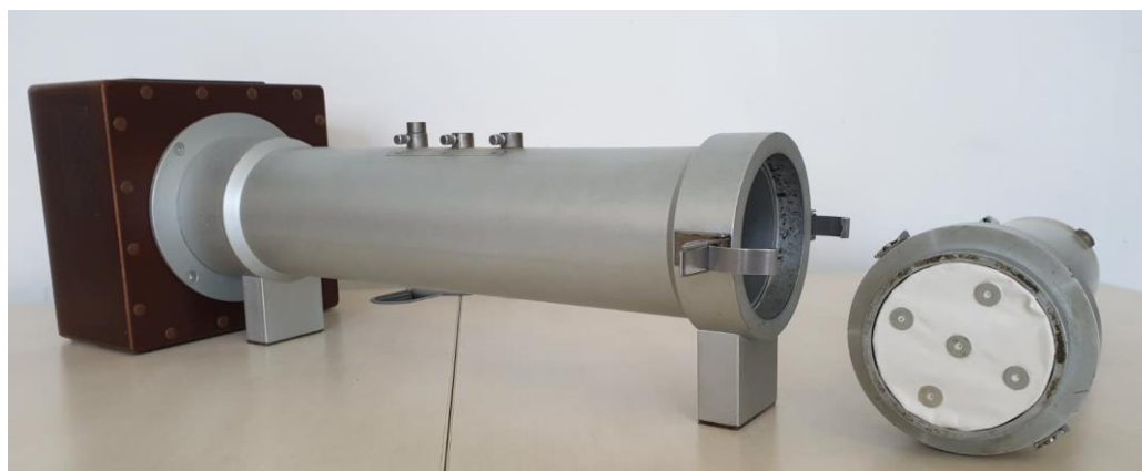
Figure 4. Impedance tube for measuring the absorption coefficient at normal incidence, with the specimen housed.
