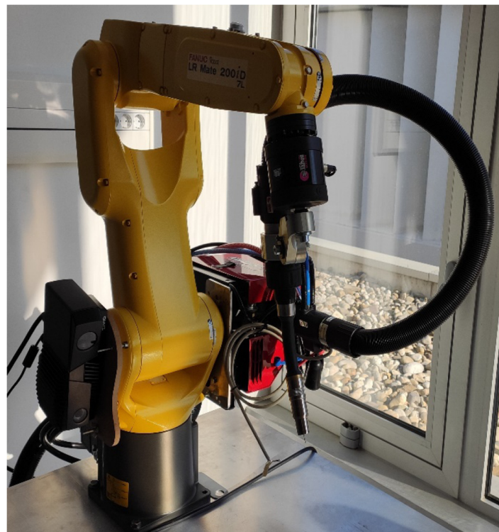
Figure 2 Robot Fanuc LR Mate 200 id/7L with Zivid One+ M structured light cam anchored
