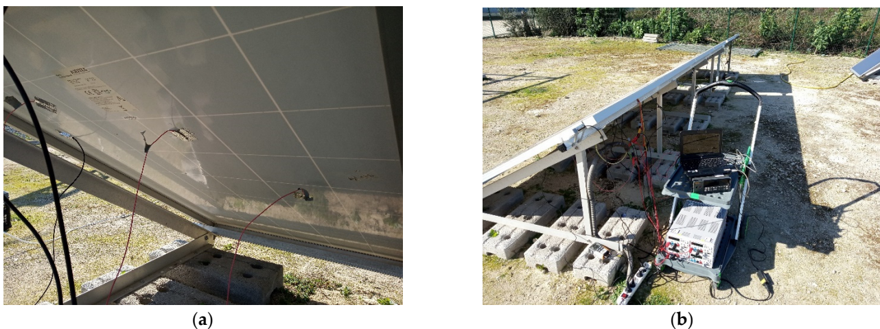
Figure 2. Contact temperature measurement method (a) Thermocouple mounting on the rear side of the module; (b) Data logging equipment.
