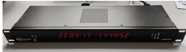
Figura 5.8: Servidor NTP local GMR5000 de *Masterclock Inc.*
