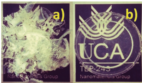
Fig. 12.1 (a) Photograph of the commercial consolidant Tegovakon and (b) photograph of a xerogel prepared by the developed route
