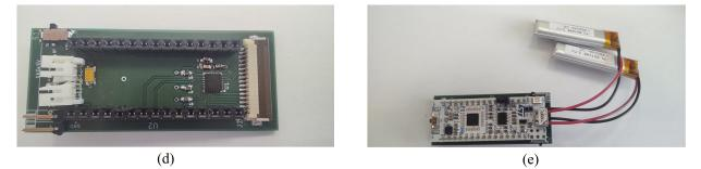
Figure 4. Prototype components: (a) PDM-based dielectric layer; (b) flexible PCB with remaining photoresist ink, prior to copper-dissolution step; (c) the insole with three layers finished, prior to fixing them with Kapton; (d) ACShield built to house the CDC Controller Ad7147-1 and to connect both plantar insole, batteries, bluetooth and MCU to the whole system; (e) ACShield with MCU and batteries connected.
