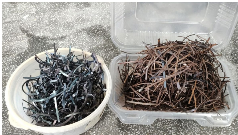
Figure 2. Pre and post - surface treatment of oxidation to steel shavings.
