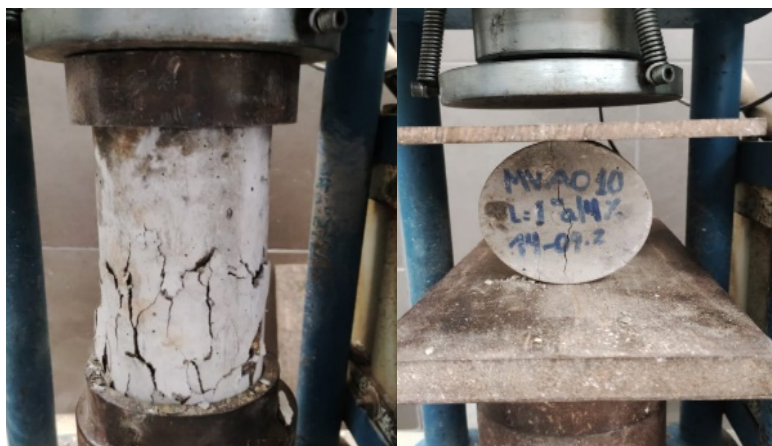
Figure 4. Compressive and indirect tensile failures.
