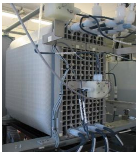
Figure 4: Stack of the VRFB and its reference cell.
