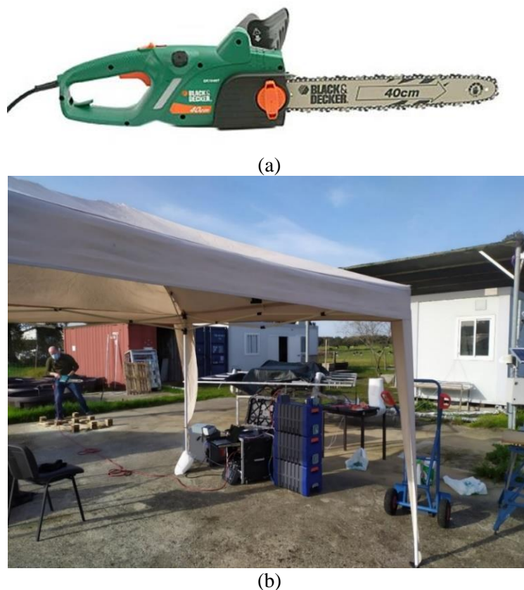
Figure 41. a) Electric chainsaw used as a representative load, and b) chainsaw exterior use-case test.
