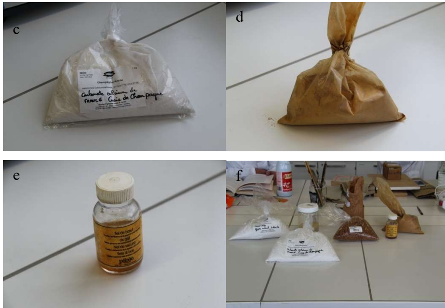
Figure 4.1 Materials used for the development of the paint model replicas: a- Bone glue, b- Gypsum sulphite, c- Calcium carbonate, d- Yellow ochre, e- Linseed Oil, f- overview of materials
