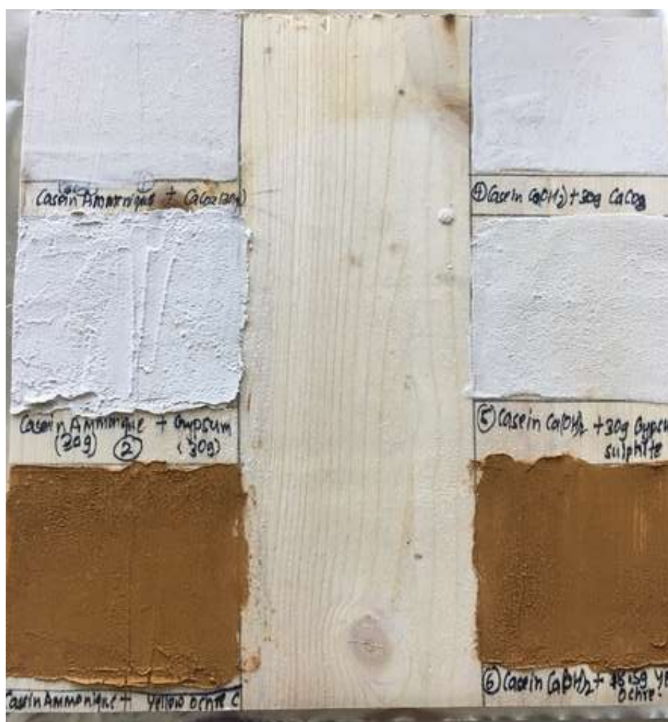
Figure 4.9 Representation of Paint models for casein and their preparation
