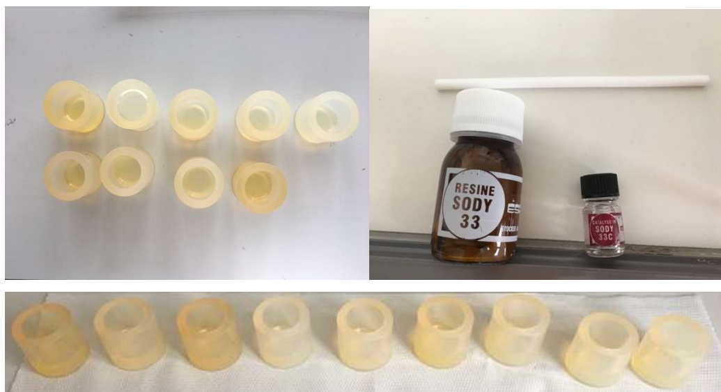
Figure 1.1 Selection of the moulds and the Resin used for the sample preparation
