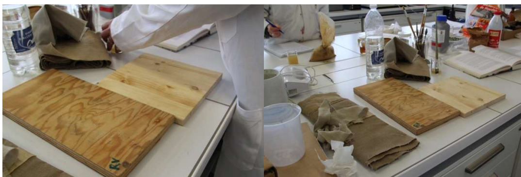
Figure 4.2 Supports for the proteinaceous paint models
