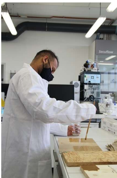
Figure 4.4 Initial layer of animal glue on the supports
