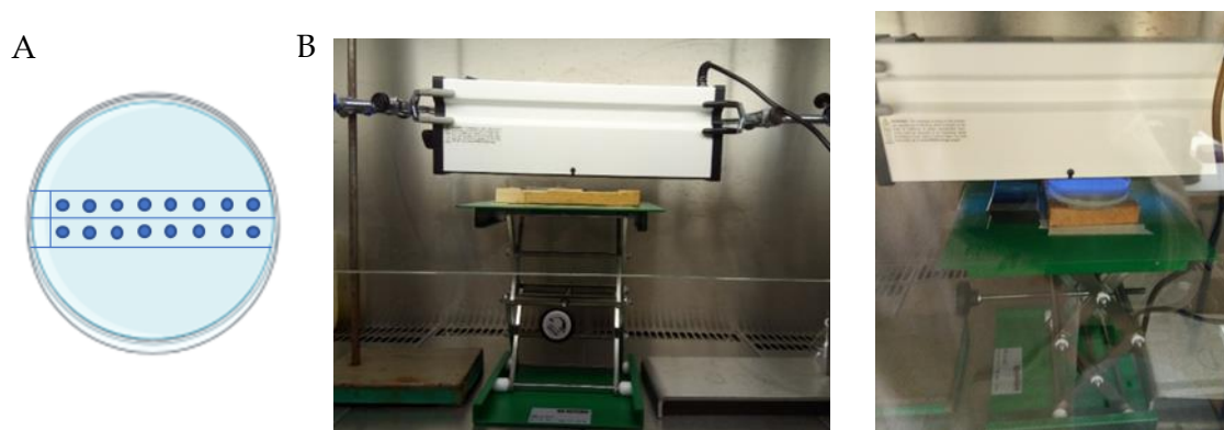
Figure 3.4 - Scheme of the UV-C assays. The plate with the drops with different dilutions (A) and the set up assembled in the laminar flow chamber (B).
