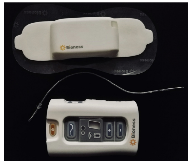
FIGURE 3: Image of a percutaneous PNS showcases the 3 components of the system: the external pulse transmitter (EPT) and electrode patch, the implanted lead, and the patient programmer. Top The EPT on top of the electrode patch. Whenever the patient wishes to trigger stimulation for pain relief, she places the electrode patch on her forearm's skin directly overlying the trajectory of the implanted lead. The EPT is then attached to the electrode patch, delivering neuromuscular electrical field stimulation through the electrode patch to the implanted lead. Middle One of the leads that was implanted parallel to the patient's left median nerve. Bottom The patient programmer, which the patient and the medical staff utilize to adjust the stimulation parameters after implantation.
