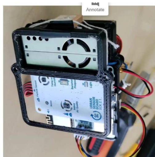
Fig. 1: Hardware consists of environmental sensors and a GPS antenna.
