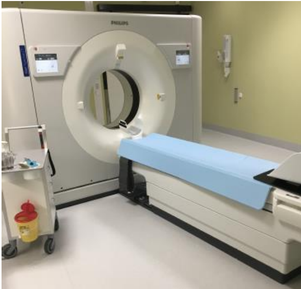
Figure 3. A dual-layer detector DECT system at Karolinska University Hospital. On the outside, conventional CT and DECT systems have a similar appearance.
