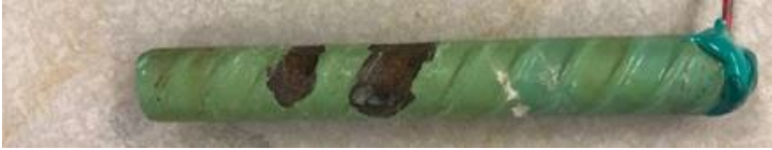
Figure 3.18: Specimen ECR1-UV-1000-4 anode after disbondment test
