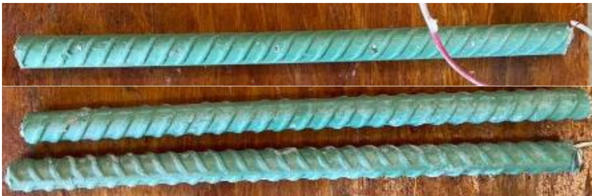
Figure 3.62: Top bar (top) and bottom bars (bottom) of specimen CB-ECR1-3 after 96 weeks of testing
