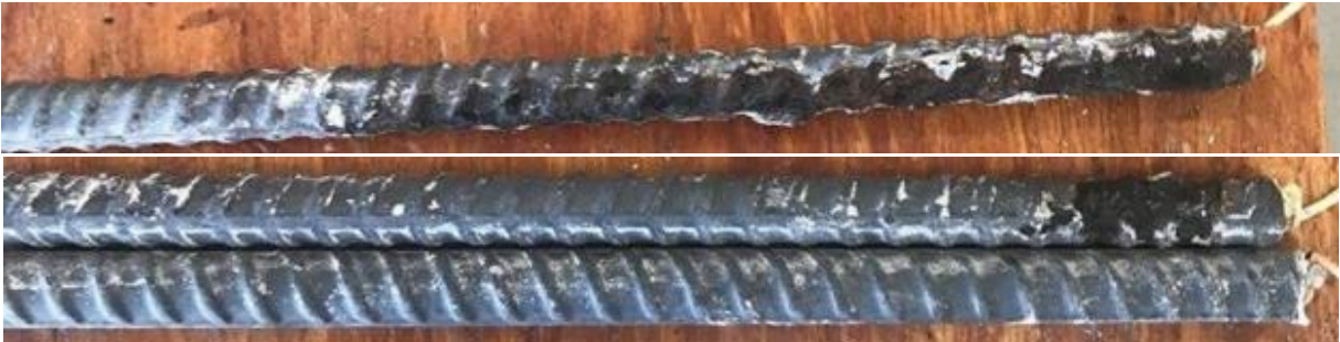
Figure 3.82: Top bar (top) and bottom bars (bottom) of specimen CB-ChromX-IPANEX-6 after 96 weeks of testing
