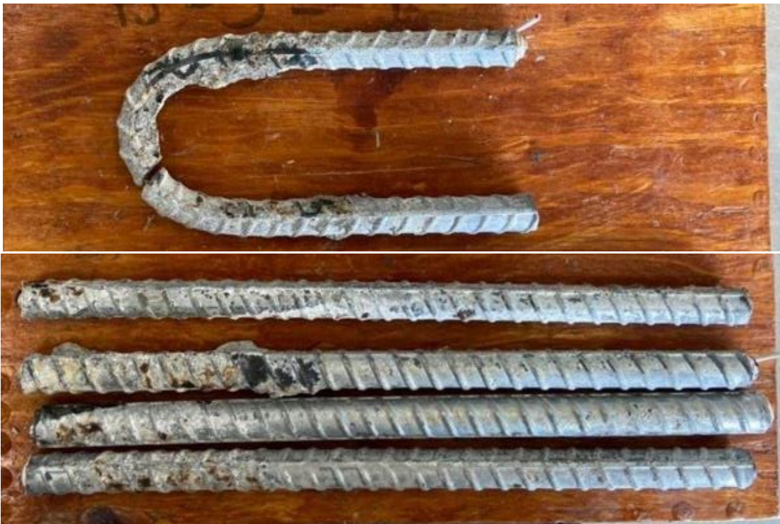
Figure 3.77: Top bar (top) and bottom bars (bottom) of specimen SE-Bent-A1094-2 after 96 weeks of testing
