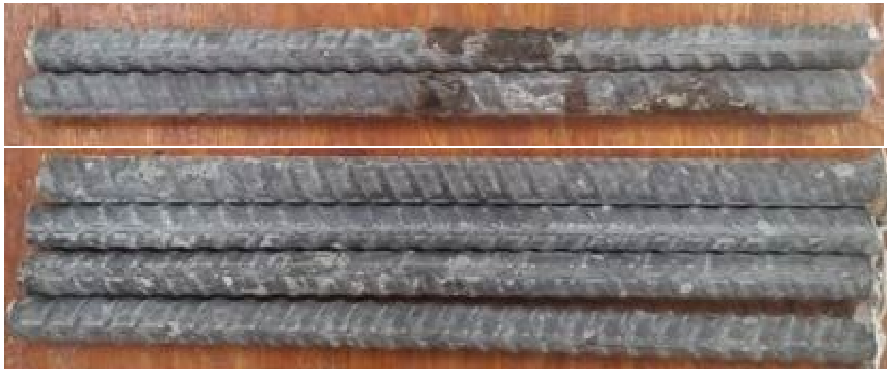
Figure 3.80: Top bars (top) and bottom bars (bottom) of specimen SE-ChromX-Xypex-1 after 96 weeks of testing
