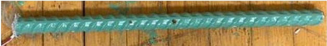
Figure 3.65: Top bar of specimen CB-ECR1-ND-1 after 96 weeks of testing
