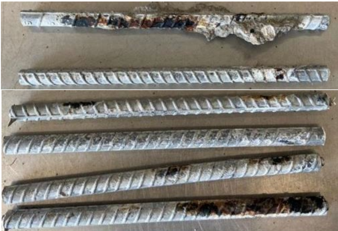
Figure 3.74: Top bars (top) and bottom bars (bottom) of specimen SE-A1094-4 after 96 weeks of testing
