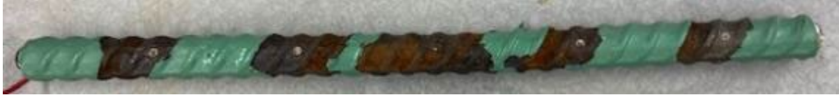
Figure 3.63: Top bar of specimen CB-ECR1-2 after disbondment test
