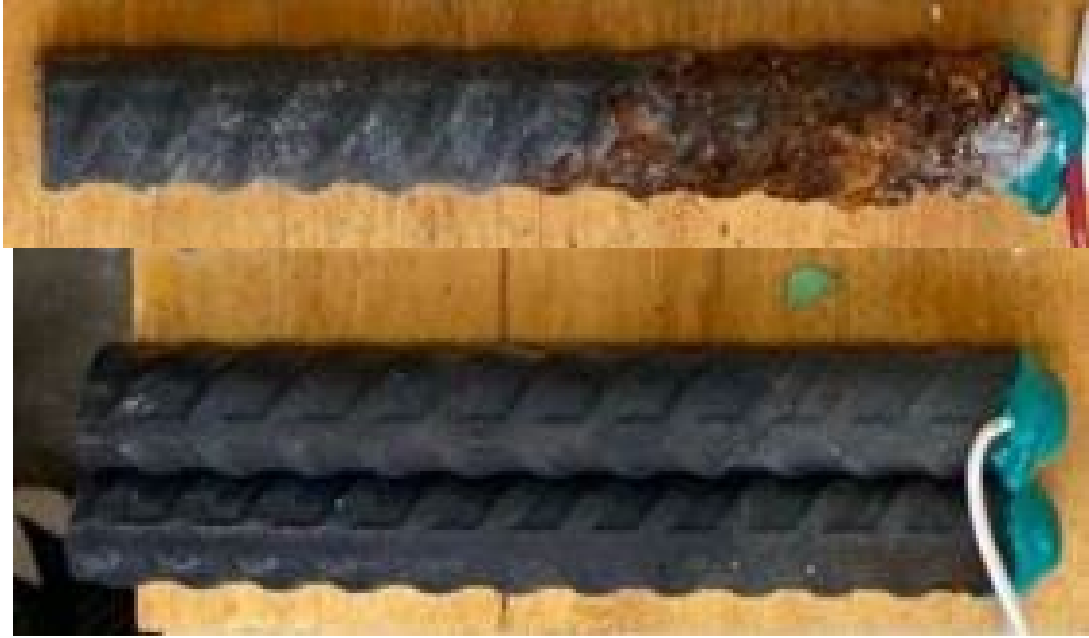
Figure 3.23: Specimen ChromX-6 anode bar (top) and cathode bars (bottom) after 15 weeks of rapid macrocell testing
