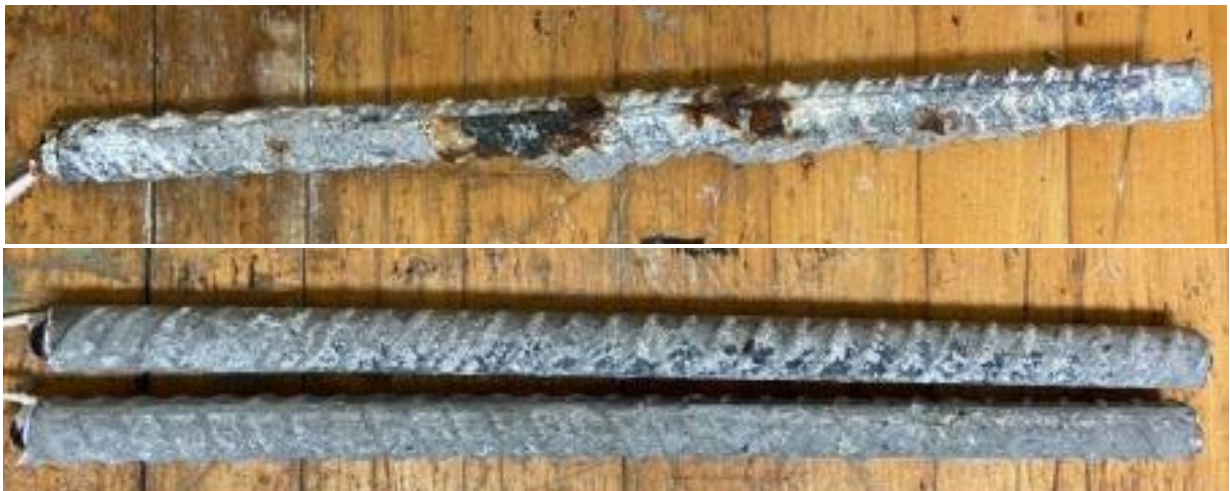
Figure 3.73: Top bar (top) and bottom bars (bottom) of specimen CB-A767-3 after 96 weeks of testing
