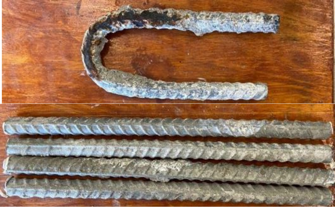
Figure 3.76: Top bar (top) and bottom bars (bottom) of specimen SE-Bent-A767-2 after 96 weeks of testing
