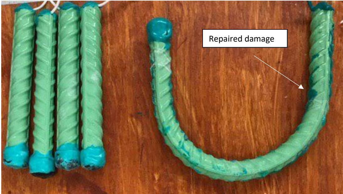
Figure 3.15: Specimen ECR1-5 anode bar (right) and cathode bars (left) after 15 weeks of rapid macrocell testing. Arrow identifying area with repaired damage
