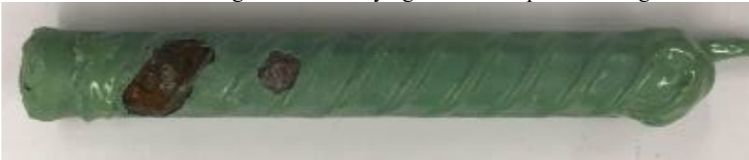
Figure 3.16: Specimen ECR1-2 anode bar after disbondment test
