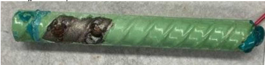
Figure 3.20: Specimen ECR2-UV-200-3 anode bar after disbondment test
