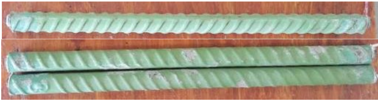
Figure 3.71: Top bar (top) and bottom bars (bottom) of specimen CB-ECR1-UV-1000-ND-1 after 96 weeks of testing
