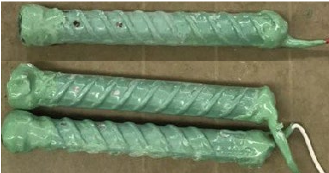
Figure 3.14: Specimen ECR1-2 anode bar (top) and cathode bars (bottom) after 15 weeks of rapid macrocell testing
