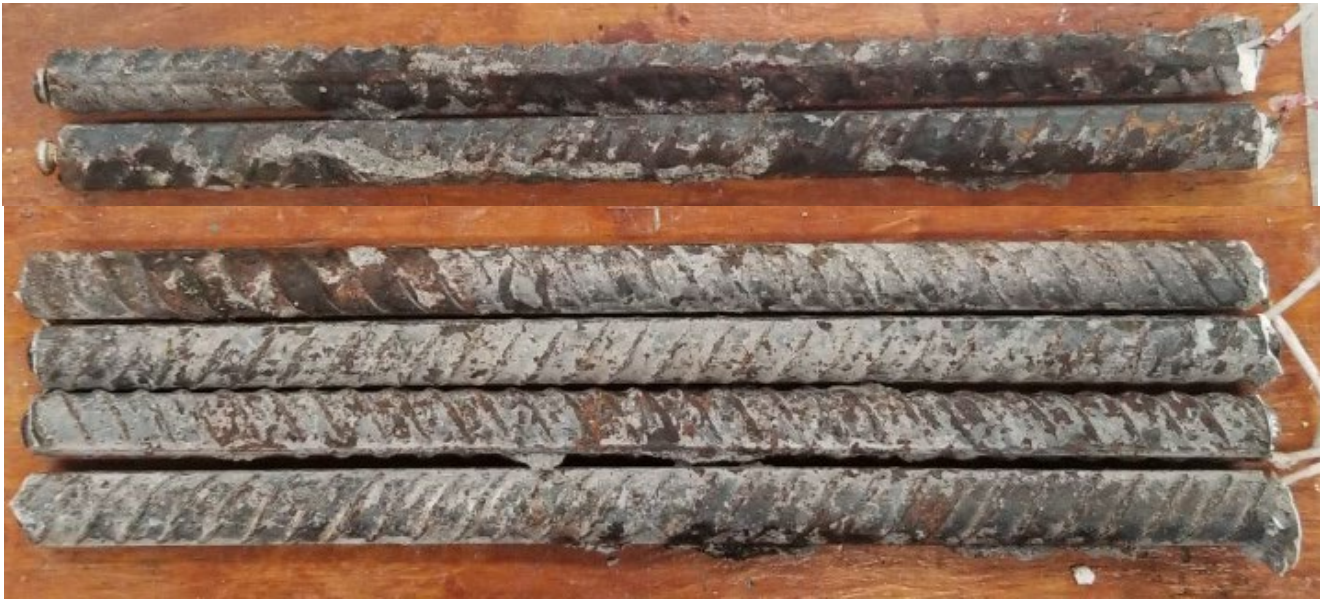
Figure 3.86: Top bars (top) and bottom bars (bottom) of specimen SE-Conv-B-Xypex-1 after 96 weeks of testing
