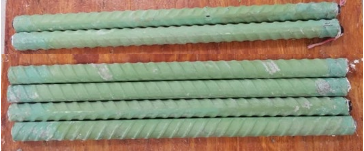
Figure 3.68: Top bars (top) and bottom bars (bottom) of specimen SE-ECR1-UV-1000-ND-1 after 96 weeks of testing
