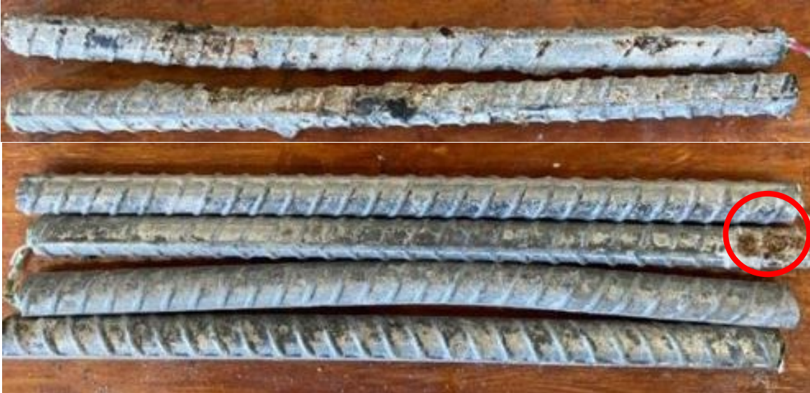
Figure 3.72: Top bars (top) and bottom bars (bottom) of specimen SE-A767-2 after 96 weeks of testing. Oval indentifying rusted region
