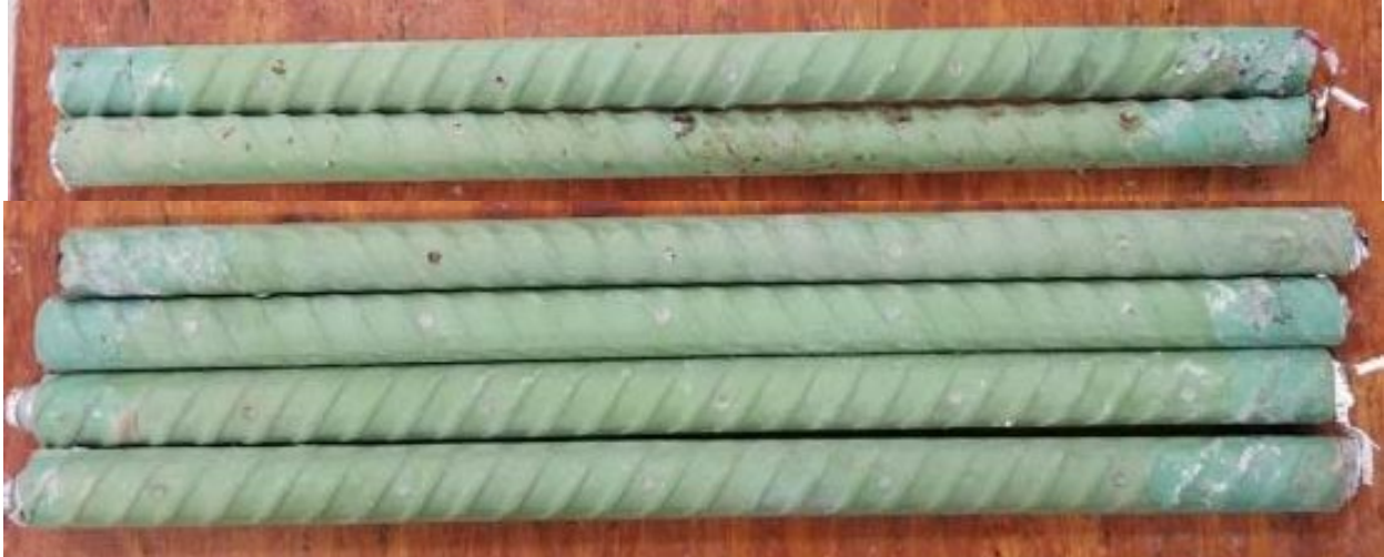
Figure 3.66: Top bars (top) and bottom bars (bottom) of specimen SE-ECR1-UV-1000-1 after 96 weeks of testing
