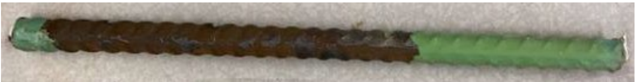
Figure 3.67: Top bar of specimen SE-ECR1-UV-1000-1 after disbondment test
