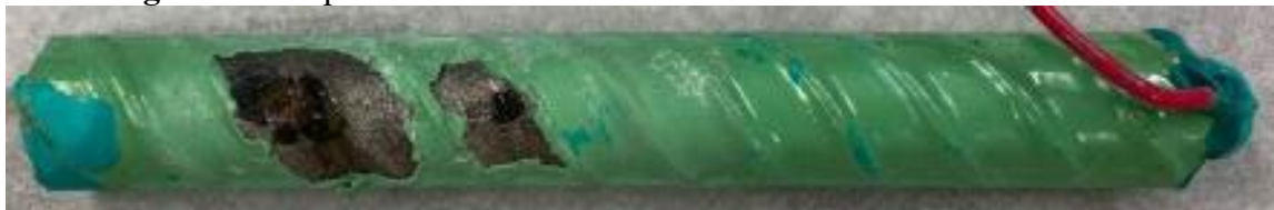
Figure 3.21: Specimen ECR2-UV-100-4 anode bar after disbondment test
