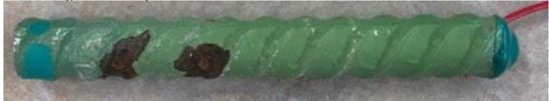
Figure 3.19: Specimen ECR1-UV-500-5 anode bar after disbondment test
