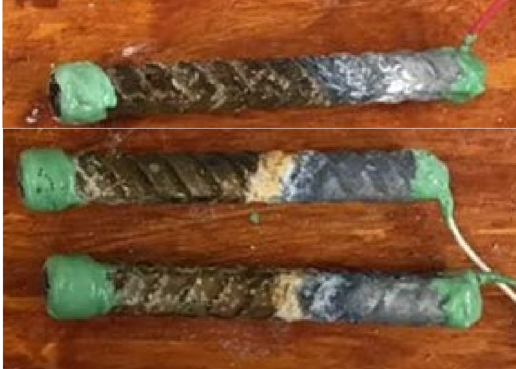
Figure 2.4: Specimen A767-1 anode bar (top) and cathode bars (bottom) after 15 weeks of rapid macrocell testing
