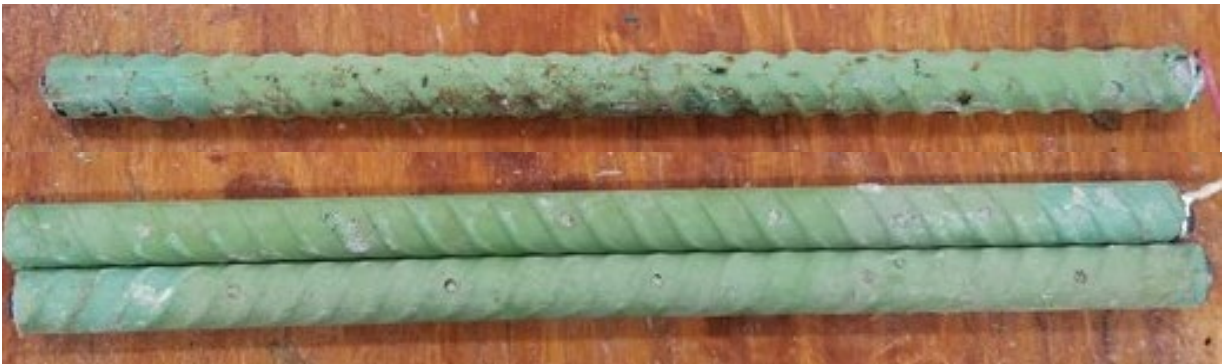
Figure 3.69: Top bar (top) and bottom bars (bottom) of specimen CB-ECR1-UV-1000-2 after 96 weeks of testing
