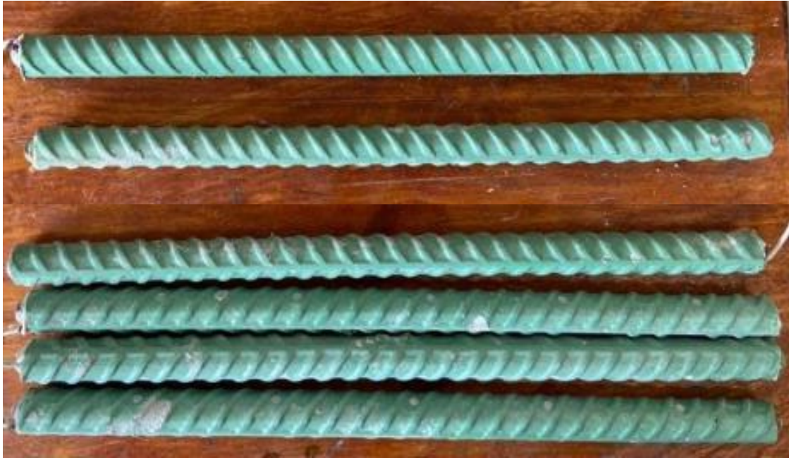
Figure 3.59: Top bars (top) and bottom bars (bottom) of specimen SE-ECR1-2 after 96 weeks of testing
