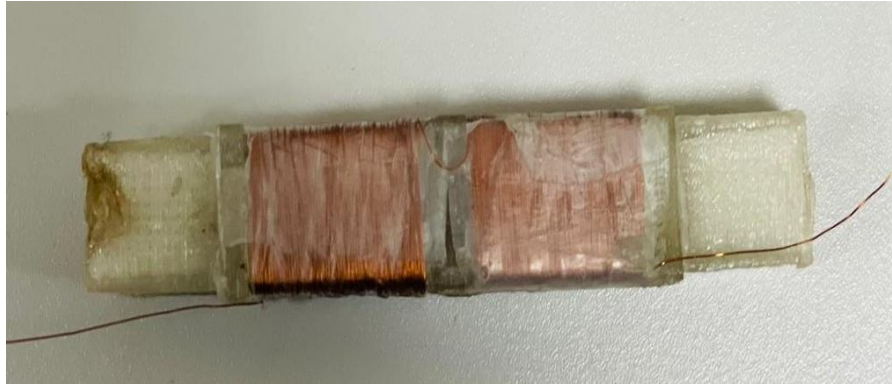
Figure 4.2. Coil wrapped around the 3D tube
