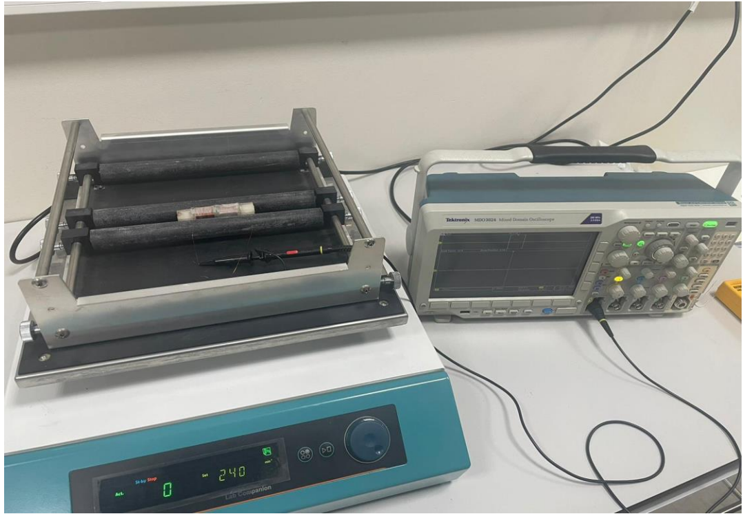
Figure 4.4. Experimental setup of open circuit voltage calculation
