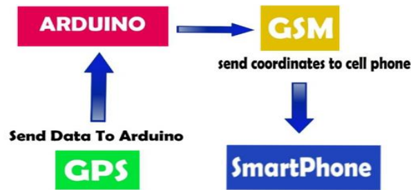
Figure 1. Block diagram of the system
