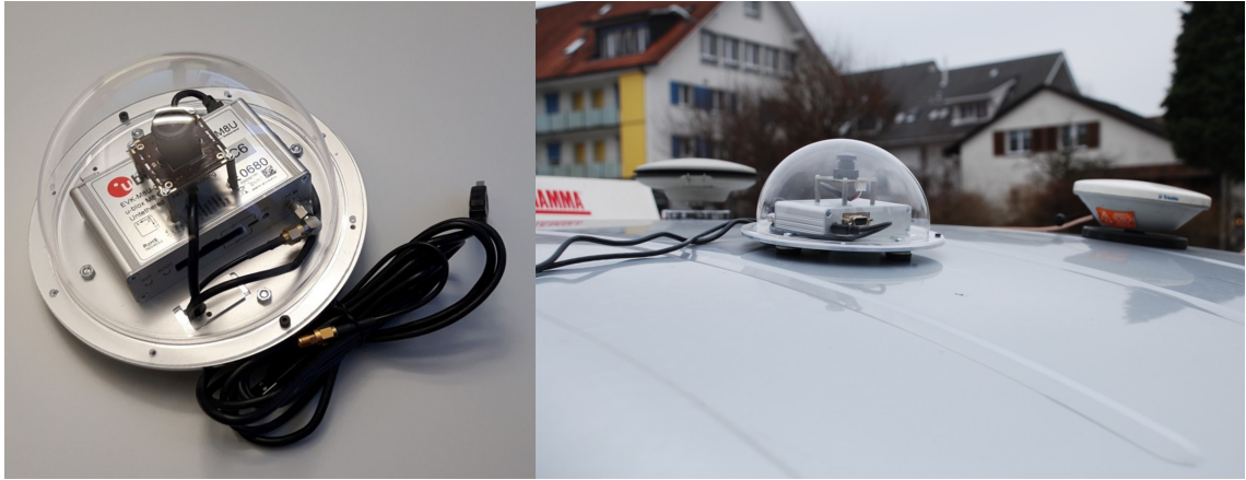
Figure 4.1. Recording setup. The fisheye camera and GNSS evaluation kit are installed on top of a van in a protective housing.
