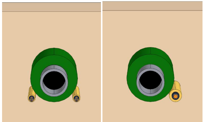
Figure 6: Buried 1 m to top of pipe with heat tracing (left) and DEH (right).
