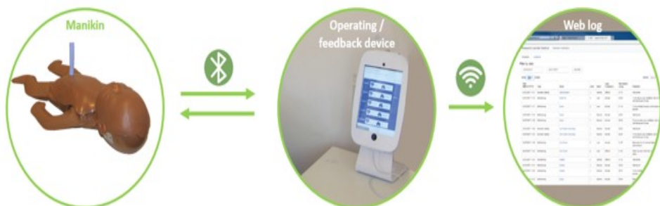
Figure 18 The manikin and NeoNatalie Live app communicate via Bluetooth. Training data from the iPad is automatically uploaded to a weblog.
