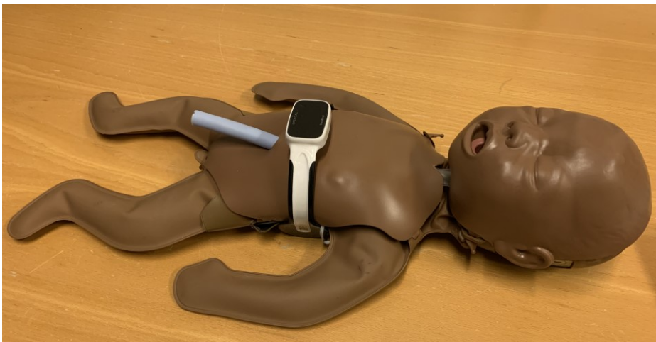
Figure 16. A NeoNatalie manikin with an attached NeoBeat heart rate meter
