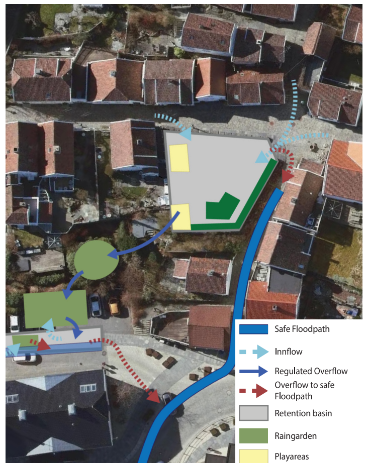
Fig. 90. The proposed solution for dividing retaining and filtering the water going through Straen into Nedre Strandgate. The floodway will be secured, choked inlets and outlets will ensure a safe water treatment (IP, 2023).
