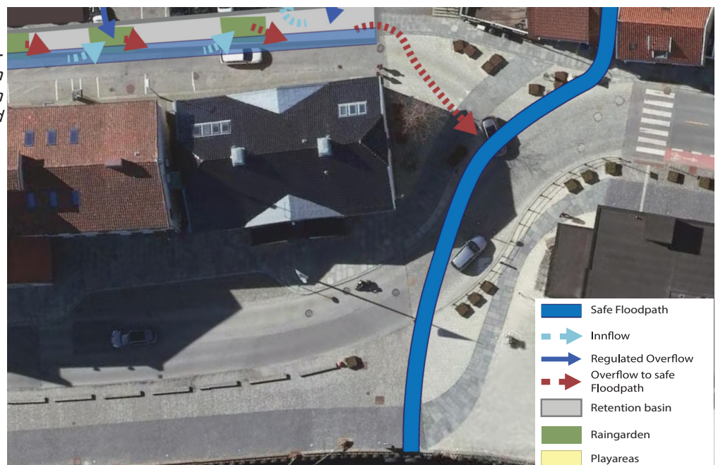
Fig. 98. Proposed solution for retaining and filtrating the water in Nedre Strandgate. the water from the floodway can be transferred into the Vågen (IP, 2023).
