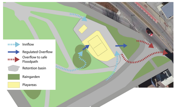
Fig. 80. Proposed rainbeds and retention basin, with inflow, choked outflow, and overflow marked (IP, 2023).
