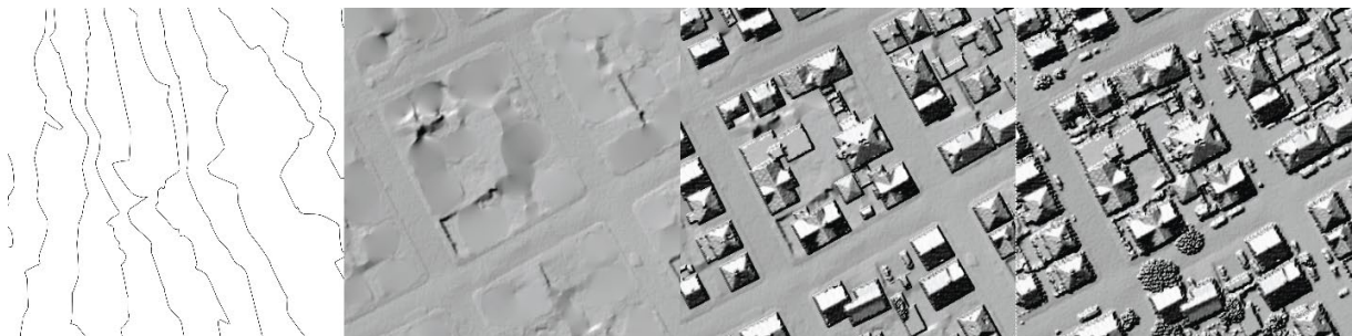
Figure 5. the same geographical area, in different map formats. From left: Contour map, DEM (Digital Elevation Model), Hybrid of DEM and DSM (Digital Surface Model), DSM
