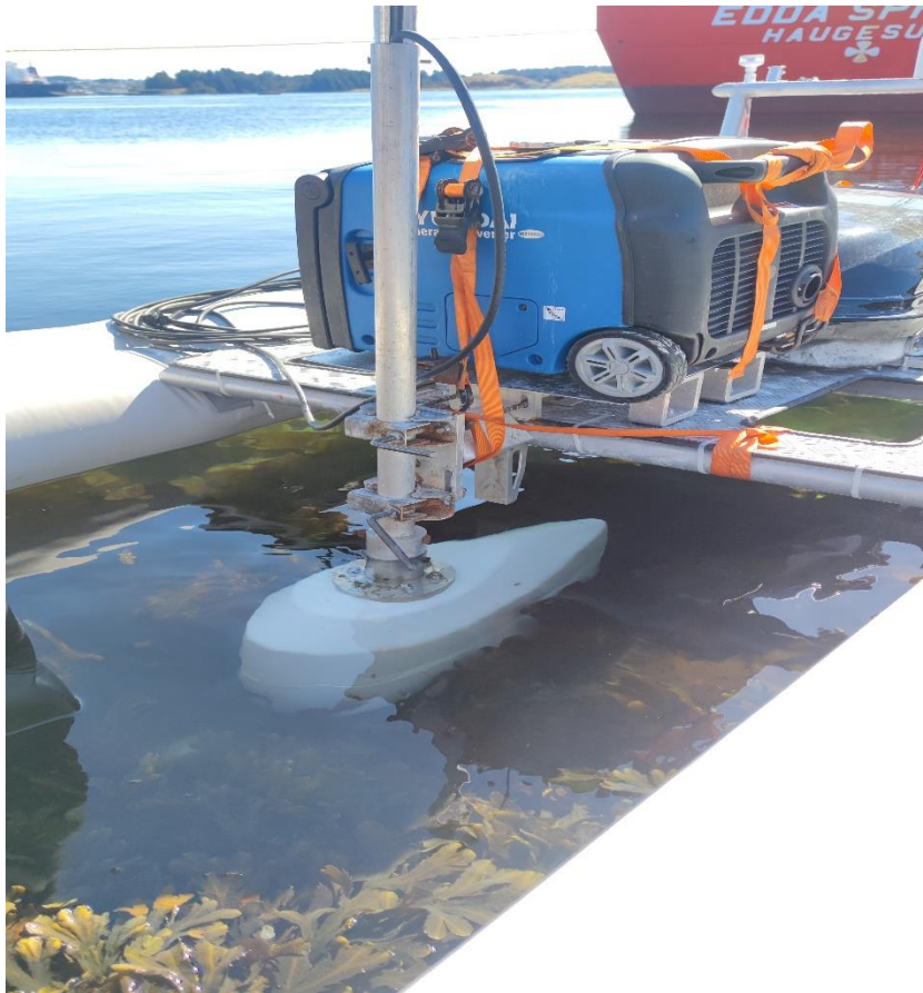
Figure 15 A close up image of the sub bottom profiler chirp
