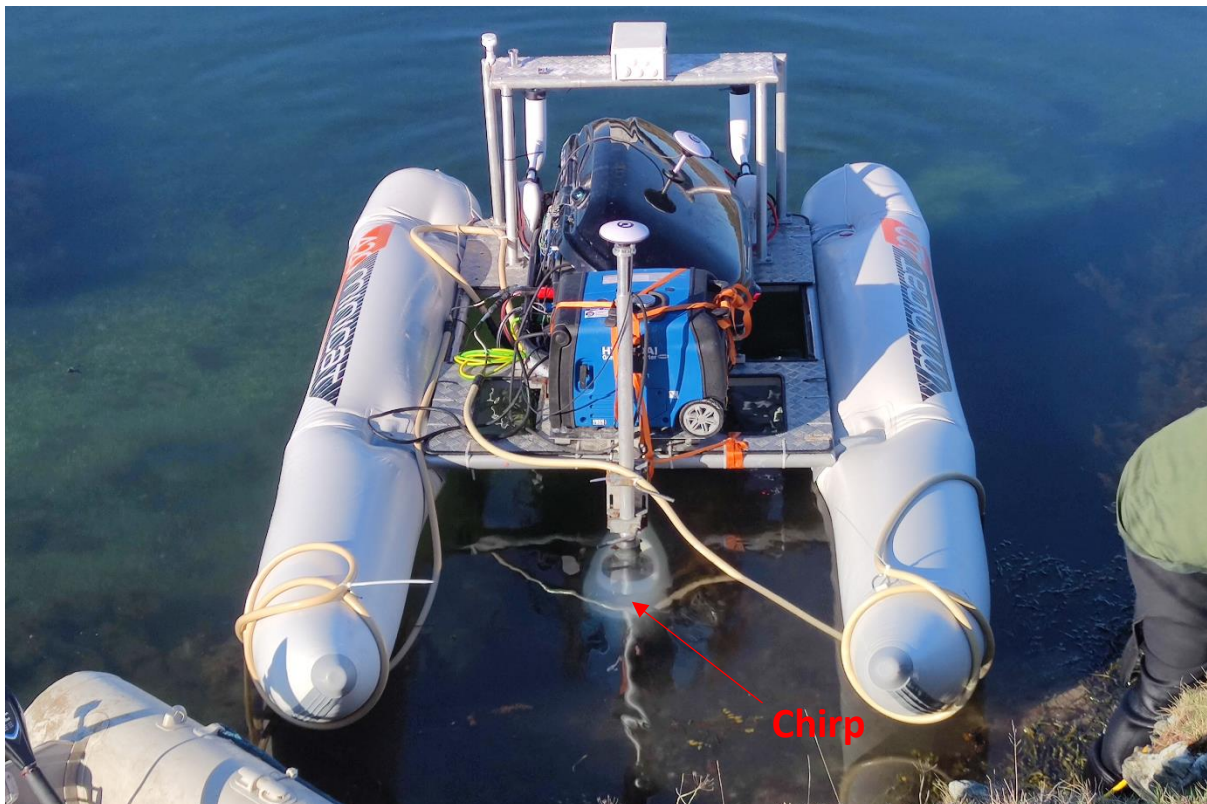
Figure 11 MERIDATA Sub-bottom profiler with a submerged chirp
