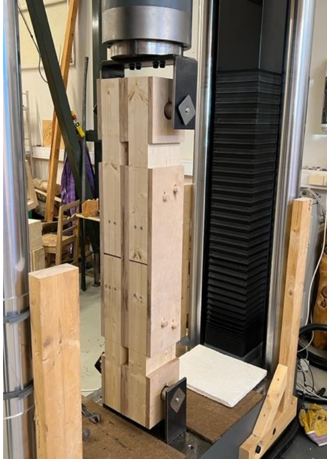
Figure 3-9 – Visual representation of how the specimens is restrained with a fully threaded steel dowel with a diameter of 50mm.
