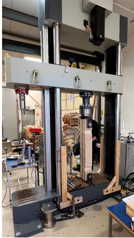
Figure 3-8 – The Zwick ZR1200 test machine with the prototype attached in it.
