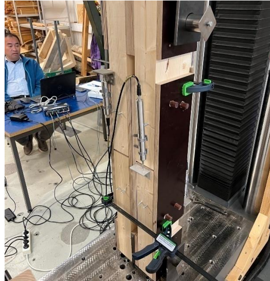
Figure 3-12 – Visual representation of how the clamps is attached to hold the plywood plates adjacent to the Glulam pieces.
