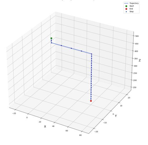
Figure 4.9: Robot Arm Trajectory. Trial: Short Rope
