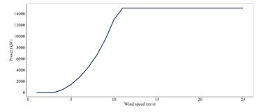
Figure 5.5: Power Curve for the 15MW\_240D reference turbine (IEA, 2020)
