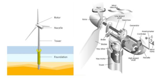
*Figure 3.14: Components of a HAWT Source: Jiang et al. (2022)*
