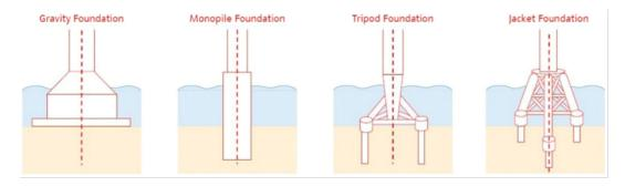
*Figure 3.16: Some bottom-fixed OW foundations Source: Liao et al. (2019)*
