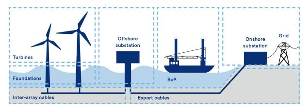
*Figure 3.17: Trivialized electricity transmission system of an OWF Source: World Forum Offshore Wind (2022)*
