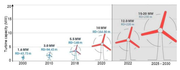
*Figure 3.15:* Development of wind turbine power and rotor diameter Source: Bošnjakovic et al. (2022)
