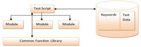
Fig. 4. Hybrid Testing Framework Schema [20]
