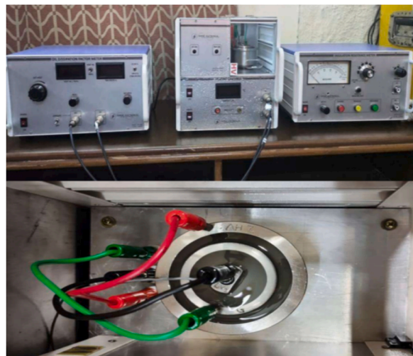
Fig. 20. I. R Tester, Oil dissipation factor meter, heating chamber and test cell for measurement of dielectric constant.
